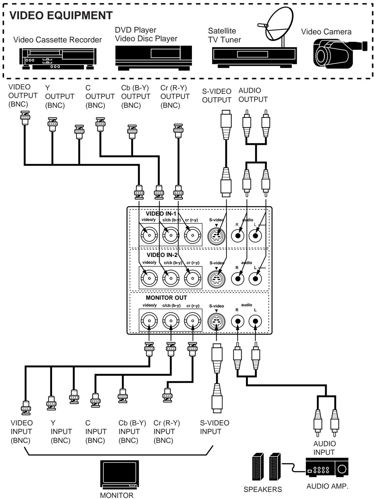
NOTE: The hook up should be done as per the above illustration. After hook up, turn on the projector, video equipment, in that order.
