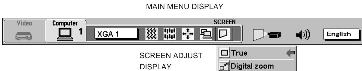
4. To adjust the image size or pan the image, move the arrow to Digital zoom by pressing POINT UP/DOWN BUTTON(s) and then press SELECT (REAR CLICK) BUTTON. MAIN MENU DISPLAY and SCREEN ADJUST DISPLAY will disappear. The "D.zoom" and the magnifying-glass icon is displayed to indicate Digital zoom mode.
