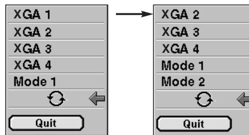
When the mark (⌂) is displayed as BLACK, computer system mode will be available on the next page. Move an arrow to the mark (⌂) and press the SELECT (REAR CLICK) BUTTON to show computer system mode described on the next page.
