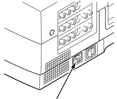
Connect the AC power supply cord (supplied) to the projector. The socket-outlet must be near this equipment and must be easily accessible.
