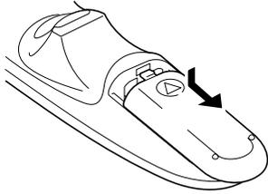
**2** Slide the batteries into the compartment.
