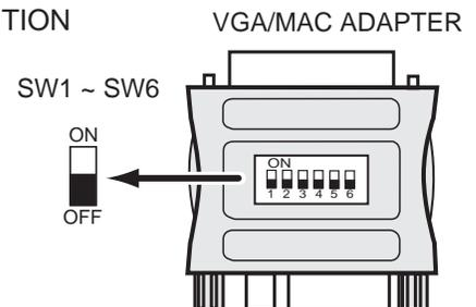
**NOTE:** The hook up should be done as per the above illustration. After hook up, turn on the projector, monitor, computer, in that order.
