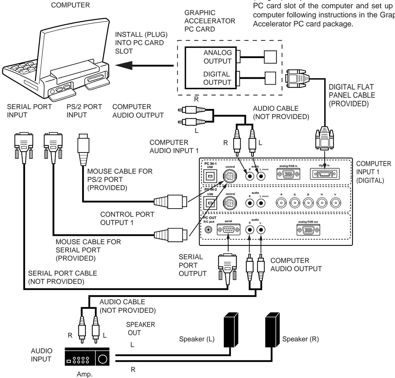
**NOTE:** The hook up should be done as per the above illustration. After hook up, turn on the projector, computer, in that order.
