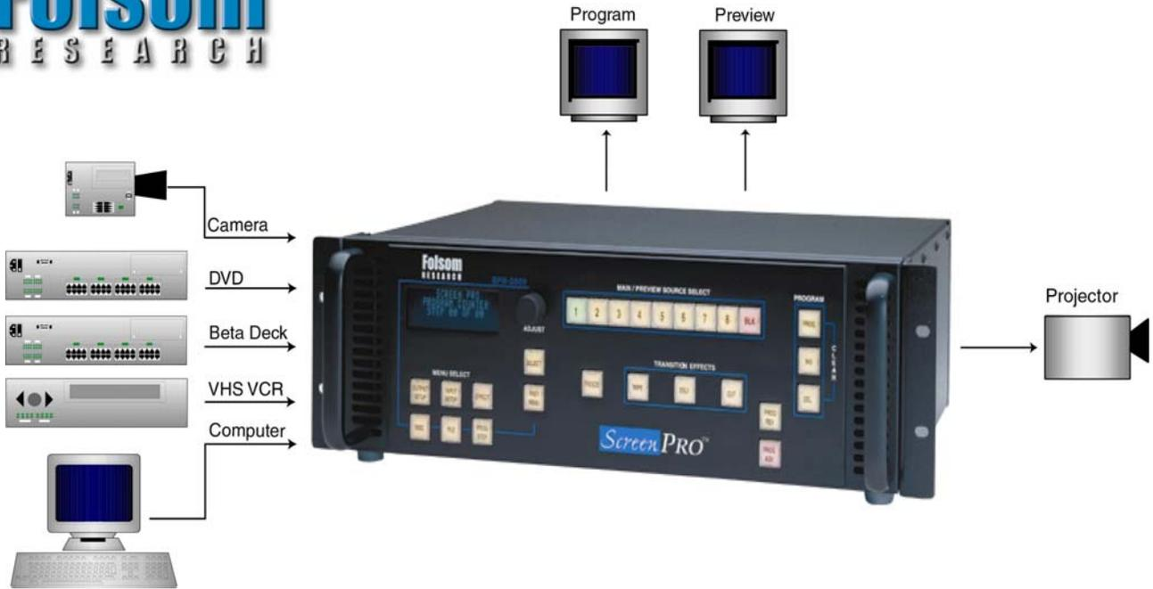
**Illustration of Typical ScreenPro™ Setup**
